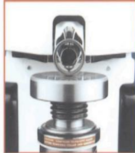
Measuring of the inner contact surface of a bearing's outer ring
