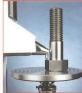
Measuring of the contact surface of a high strength screw
