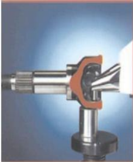
Measuring of the inner contact surface of a cardan shaft driver
