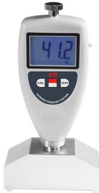
Digital Screen Tension Meter
