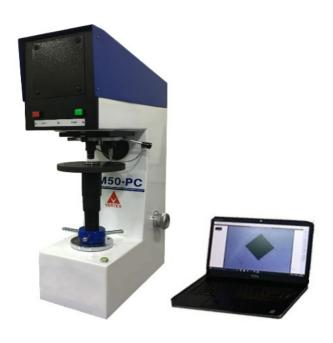
VERTEX Computerised Vickers Hardness Tester is a simple and accurate means to produce and measure the diamond indentation. The Indentation can be measured by Auto measure option given in Software there are four options to measure indentation No. 1) Remote Auto 2) Auto 3) Semi Auto 4) Manual measurement Manufacturing standard conforms to IS: 1754, ISO 6507-2 & ASTM E92
