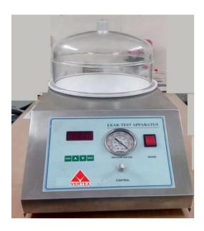
This apparatus is an ideal instrument to check sealing integrity of Blister Packs; Strip Packs; Sachet and Pouch Packs etc. It is also used for checking leaks from Capped Bottles; Induction Sealed Containers; Sealed or Crimped Tubes etc. The old method of separate desiccator and huge vacuum pump is replaced with this new Leak Test Apparatus in GMP Stainless Steel body with phenomenal compactness.
