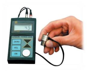
Used for measuring thickness and corrosion of pressure vessels, chemical equipment, boilers, oil storage tanks, etc. in industries of petroleum, shipbuilding, power station, and machine manufacturing. Materials measured: any hard materials, including steel, cast iron, aluminum, red copper, brass, zinc, quartz glass, polyethylene, PVC, gray cast iron, nodular cast iron and other ultrasonic wave well-conductive materials.
