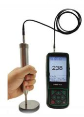
TIME5630 ultrasonic hardness tester can nondestructively measure the metals and alloys with a minimum thickness of 3 mm. It can measure strip/plate workpiece, mold hardened layer, blade hardened layer, tooth surface hardened layer, flange edge, wheel, turbine rotor, thin plate, shaft and pipe, container, knife edge, welding part, etc.
