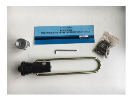
This instrument is based on a new but proven constant loading system which produces clear impressions capable of indicating accurate results whether applied statically or dynamically. Loading is guaranteed constant due to a precision pin shearing off under impact.
