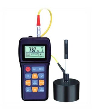
Portable Metal Hardness Testers are small and light in shape but it is very useful instruments mostly used for heavy metal parts where we can not able to move the part from one place to another. It is mostly suitable for testing of heavy, big outdoor metal parts. it confirms to ASTM A956. They can measure in HLD, HV, HB, HRC, HRB & HS they can measure up to 68 HRC and up to 955 HV.
