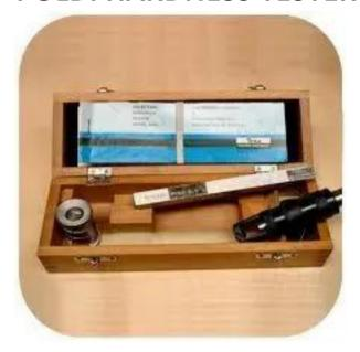
The hammer type Poldi impact hardness tester is useful for simple and quick determination of Brinell hardness of metals such as steel, Cast Iron, Brass, Aluminum, Copper etc. Due to easy handling and maneuverability, this tester is most suitable for testing heavy castings and other components.
