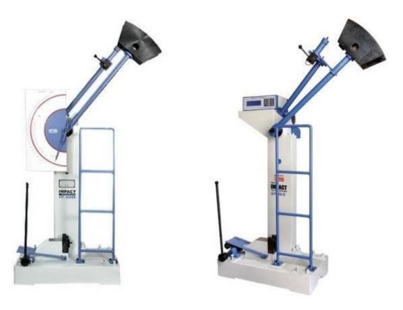
The pendulum Impact Tester Model IT 30 is designed for conducting Izod, Charpy test. The test methods confirm to
