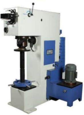
VERTEX make optical Brinell Hardness Testing machine is a production testing Machine. Operation of the machine is similar to the VB 3000. Swiveling mechanism of the ball indenter, Built-in optical systems with 14 x magnification & projection screen with micrometer of least count 0.01 mm are the additional features of this machine. This helps the operator to measure the impression directly on the screen without moving the job. This machine confirms to IS: 2281 / 1983 and BS 240.
