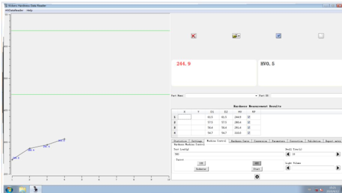
Software can control the machine turret and generate test report including hardness value curve. Software install on the computer, connect with hardness tester through RS232 port. All the testing result can save to computer and generate test report in word format.
