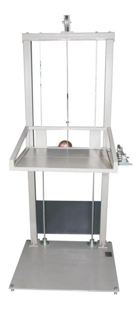
This instrument performs a vertical impact test on a complete, filled transport package by dropping as per **IS/ASTM/ISO/DIN** standards. The test may be performed either as a single test to investigate the vertical impact or as a part of a sequence of tests designed to measure the ability of a package to withstand a distribution system that includes a Vertical Impact hazard.
