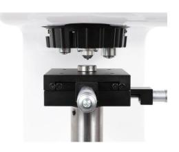
Automatic turret design, Loading - Dwell - Unloading automatically process, greatly improved machine accuracy and working efficiency.
