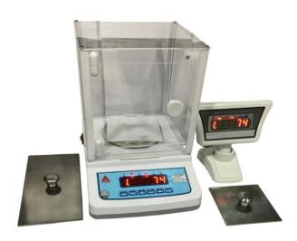
This equipment measures and directly indicates substance in terms of grams per sq. meter (GSM). It displays GSM of samples cut selected to size on a digital indicator, very useful to measure Paper, Paper Board, Fabrics, Plastic Films, Leather, Aluminium foils & Fibre sheets.
