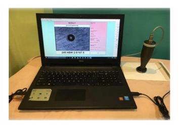
This is automatic Brinell microscope. The specially developed software gives reliability & repeatability in Brinell measurement.
