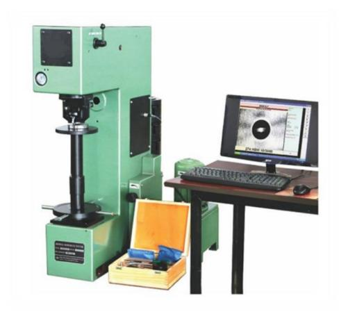
Computerized Brinell Hardness Tester is a simple and a accurate means to produce automatically measures the ball Indentation give Brinell hardness number. These testers are suitable for measuring the hardness of metallic parts with wide lasting range - from soft to hard, and their accurate results are widely acclaimed. These testers strictly confirm to IS: 2281, BS: 10003-2 and ASTM E-10.
