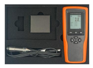
These gauges can be used for non-destructive coating thickness measurement of non-magnetic coatings, e.g. paint, enamel, chrome on steel, and insulating coatings, e.g. paint and anodizing coatings on non-ferrous metals.
