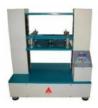
This equipment is designed to measure the ability of the container to resist external compression loads during transit and storage. Compression Strength Test also serves as a useful index of overall quality of the material and workmanship of the box.
