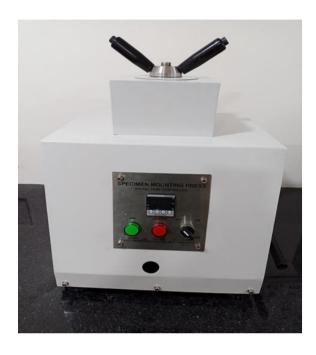
The mounting press is equipped with a digit temperature controller to establish real-time temperature meanwhile, a timer is equipped to realize the Automatic of sample making while obviously increasing working efficiency. For each specimen-mounting 3-4 minutes is enough and a mirror-like specimen can be acquired, High speed mould heater with built-in water-cooling coils. Interchangeable mould. Suitable for high volume application, relieves operator fatigue
