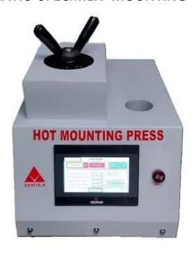
The mounting press is equipped with a digit temperature controller to establish real-time temperature meanwhile, a timer is equipped to realize sample making Automatically increasing working efficiency. For each specimen-mount making 3-4 minutes is enough and a mirror-like specimen can be acquired, High speed mould heater with built-in water cooling coils. Interchangeable mould. Suitable for high volume application, relieves operator fatigue
